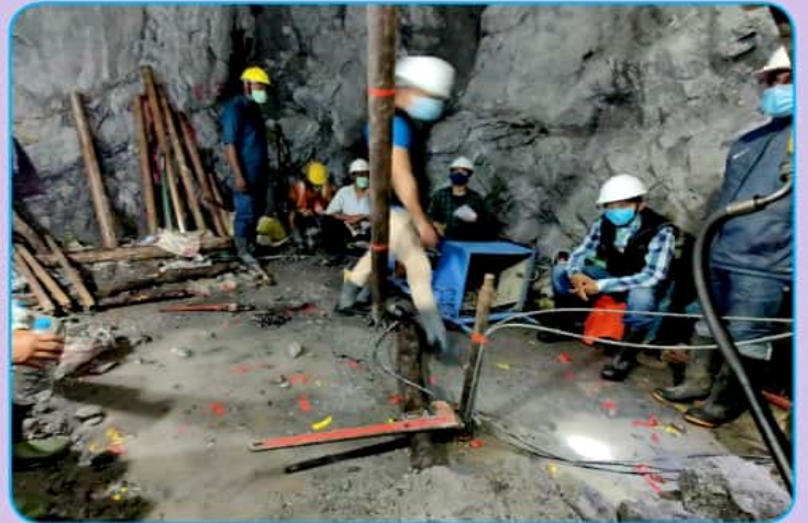
Hydro-fracture Test inside Tunnel
