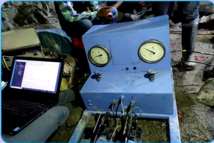
Hydro-fracture Test inside Tunnel
