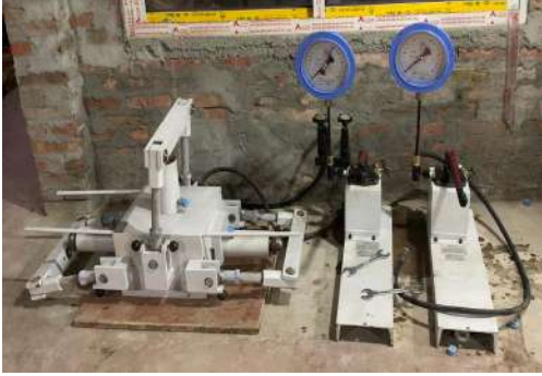
Fig. Direct Shear Testing machine (Rock)
