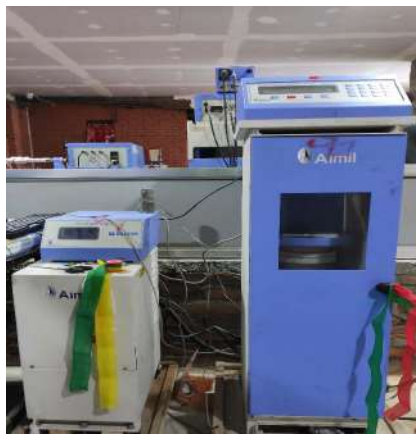
Fig.: Automatic Compression Machine for Modulus of elasticity, Poisson's Ratio and UCS
